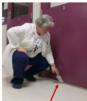
Tissue test: Place tissue outside door and see if it gets sucked into the room
